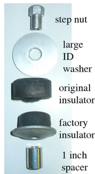
B. Assemble above parts in order shown
