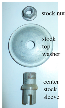
A. Remove nut, washer, and center sleeve shown above
