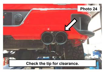
23. Adjust as necessary and tighten all clamps.
