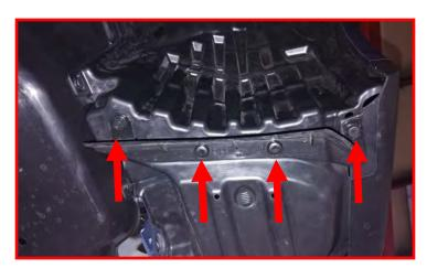
Remove all remaining plastic push clips from the inner fender liner. There are 4 clips. Save all clips. Note that the liner sits under and over the bumper cover. This will be changed later. Remove 1 plastic push clip from the lower skid plate and bumper cover.
