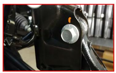
Install the brake line bracket to the strut body. Rotate the brake line bracket as shown. Originally the brake line was bolted from the bottom upwards to the strut, now it will be mounted to the top of the strut body using the factory hardware. Torque to 5 ft-lbs. Make sure to rotate the ferule inside the cut out on the strut body. Refer to disassembly step for reference if needed.
