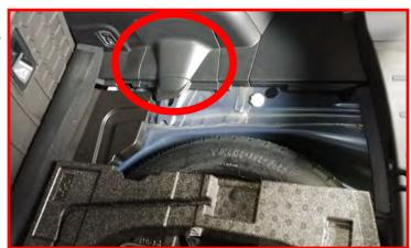
Remove the strut nuts and set aside.
