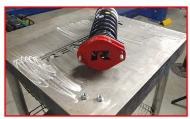
Install the completed strut assembly to the car using the provided M10 flange nuts. Do not tighten at this time. A helper is recommended.
