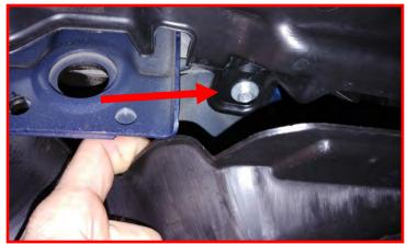
Take the plastic liner and install above the bumper cover. You will see one ear of the bumper cover that originally sits under the liner, this needs to be relocated to the outside of the liner.
