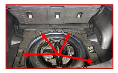
Remove these clips and set the foam pieces aside. Remove the strut covers by pulling upwards at the trunk area, then pushing down at the plastic cover, and set aside.
