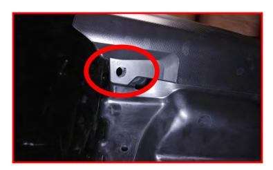
Finish off the liner movement by pushing forward 1". Mark and drill out the new plastic push clip locations. Install the remaining push clips.
