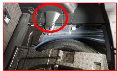
Remove the strut nuts and set aside.
