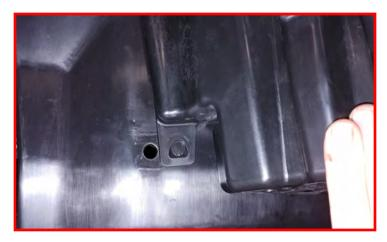
Once the liner is moved forward, use a suitable razor knife and trim the outer bumper cover edge valance. Cut straight down to the 90 degree turn, then cut at a 45 degree to the liner. The plastic is very easily cut, so take care to not slip. This can be trimmed more if necessary. Test fitment of the wheel and tire combo is recommended and trim as necessary.
