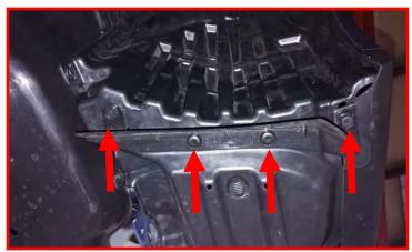
Remove all remaining plastic push clips from the inner fender liner. There are 4 clips. Save all clips. Note that the liner sits under and over the bumper cover. This will be changed later. Remove 1 plastic push clip from the lower skid plate and bumper cover.
