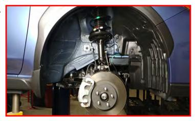
Remove the front sway bar end link at the strut body. This step should be completed on both sides to ease in installation at later steps.
