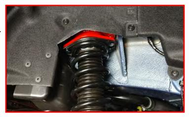
Raise the lower control arm into place and install the lower strut hardware. Do not tighten at this time. Use the jack and raise the lower control up to set pre load on the strut. Install the lower knuckle bolt. Torque to 95 ft-lbs.
