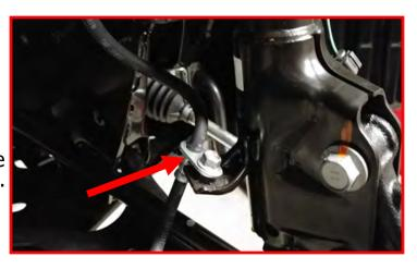
Install the ReadyLIFT sway bar bracket to the strut using the provided M12 bolts, washers, and nuts. Do not tighten at this time. If you have not started the opposite side of the vehicle at this time, you may not be able to line the sway bar up until the opposite side is released.
