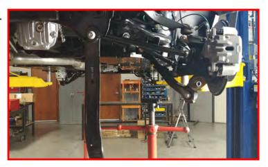
Locate the ReadyLIFT strut extension. Install using the factory hardware. You will have to start each nut before tightening fully. Run each nut down in an alternating pattern until you can torque them down. Torque to 30 ft-lbs.
