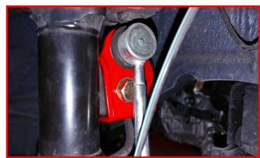
Install the front wheels and lower the vehicle to the ground. Torque the lug nuts to the wheel manufacturers specs. Jounce the front end to settle the suspension. Torque the upper strut spacers to 30 ft-lbs.
