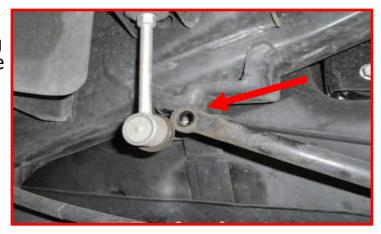
Lower the axle down enough to remove the springs and install the spacer. Be careful to not over extend any ABS or brake lines.
