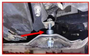
Move to the suspension, remove the sway bar end link from the knuckle. Let hang out of the way.
