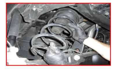
Install the ReadyLIFT spring spacer on top of the spring and rubber isolator. Install the assembly into the vehicle. Raise the axle up to hold the springs in place.
