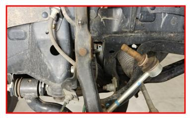
Remove the lower strut hardware.
