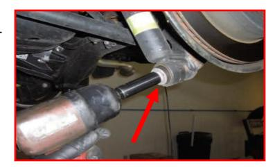
Disconnect the lower sway bar end link from the sway bar. Let the sway bar hang out of the way. Loosen but do not remove all control arms and track bar hardware.
