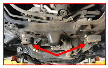
Install the ReadyLIFT differential drops in between the factory mounts and frame.
