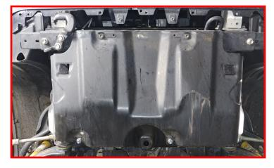
Install the rear of the front gravel guard using the provided hardware and spacers. Torque front and rear hardware to 5 ft-lbs.
