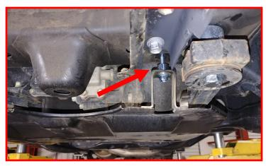
Install the front gravel guard to the core support cross member using the factory hardware. Do not tighten at this time.
