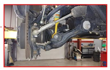
Install the sway bar end link to the knuckle using the factory hardware. Torque to 45 ft-lbs.
