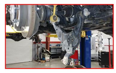
Remove the strut from the vehicle.
