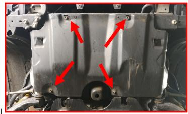
If equipped, remove the differential gravel guard.
