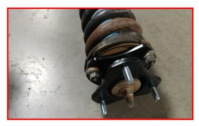
Install the completed strut assembly to the frame using the provided hardware. Do not tighten at this time.
