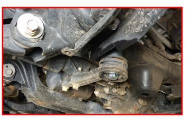
If equipped, install the differential gravel guard to the rear most cross member with the factory hardware and the front cross member with the provided hardware and spacers. Torque to 5 ft-lbs. (Driver side shown)
