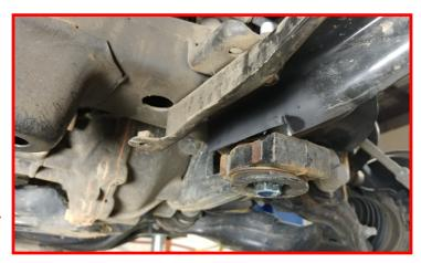
Install the previously removed passenger side gravel guard support using the factory hardware. Torque to 45 ft-lbs. (Modified mount shown)
