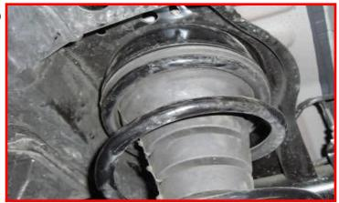
Install the shock lower hardware. Do not tighten at this time. Install the wheels and lower the vehicle to the ground. Jounce the vehicle to settle the suspension to the new ride height. Torque the lower shock hardware to 45 ft-lbs, and all control arm/ track bar hardware to 125 ft-lbs.
