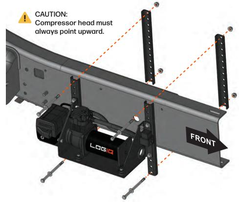
• To determine the assembly height, mock up the frame brackets around the frame as shown and position the AirlQ assembly against the frame brackets to determine which mounting holes may place the assembly in the optimum position (WARNING: If mounted low, the AirlQ Components may be at higher risk of damage from road debris and if mounted too high the compressor may transfer excessive heat to the floor).
