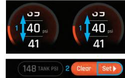
Or use the Ticker Selector by pressing one of the air spring pressure displays. Adjust the **TICKER** to the desired pressure(s) and press **>SET** in the lower right hand corner.
