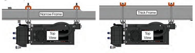
If mounting to a tall frame, use the furthest bolt holes. If mounting to a short frame, use the closest bolt holes to the height of the frame. Then cut the excess material from the bottom of the mounting brackets (paint exposed metal to avoid corrosion).
