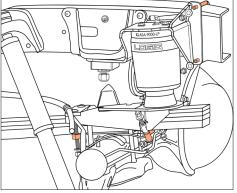
Driver assembly will be fastened with the Install the 3/8" U-bolt with washers & nuts so U-bolt and lower bracket clamps in the that it is clamping around the frame. orientation shown.
