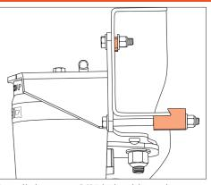
Install the upper 3/8" bolt with washers, nut and frame spacer. Ensure it is sitting flush against the frame. Install the lower 3/8" bolt with washers, nut and frame clamp. Ensure the clamp is sitting against the frame.
