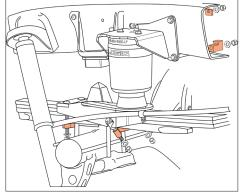
Passenger assembly will be fastened with 3/8" hardware and the lower bracket clamps in the orientation shown.
