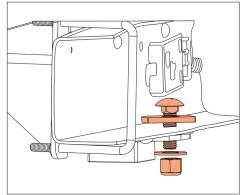
Install the supplied 5/8" carriage bolt and carriage bolt washer through the hole in the frame and the upper bracket.
