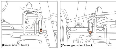
Un-bolt the emergency brake cable brackets on both sides of the truck.
