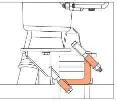
Secure the lower bracket to the leaf spring with the supplied 3/8" hardware and clamps. Make sure the bracket cut-outs are aligned with the U-bolt saddle, and the leaf spring bottom clamp is oriented correctly. Snug the hardware.
