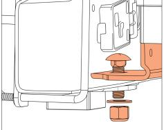
If using with an aftermarket 5<sup>th</sup> wheel bracket, install the carriage bolt WITHOUT the carriage bolt washer and instead through both the 5<sup>th</sup> wheel bracket and the upper bracket.
