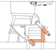
Secure the lower bracket to the leaf spring with the supplied 3/8" hardware and clamps. Make sure the bracket cut-outs are aligned with the U-bolt saddle, and the leaf spring bottom clamp is oriented correctly. Snug the hardware.
