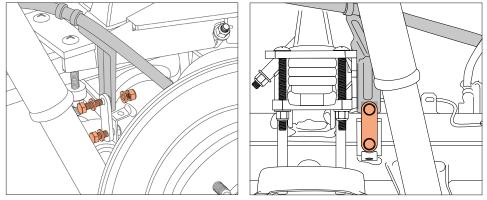
Once all fasteners are installed, use provided E-brake relocation bracket and install on driver side with provided M8 hardware. Torque to 8 FT. LB.
