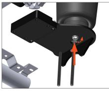
Un-bolt the 3 T40 Torx bolts holding the brake line shield to the axle to get clearance for lower bracket installation.
