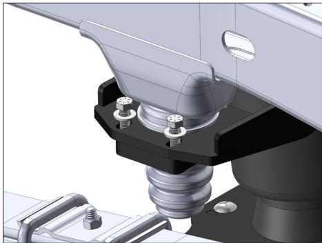
Go back to the upper bracket and install the provided 3/8" Grade 8 hardware into the bump stop spacer as shown.
