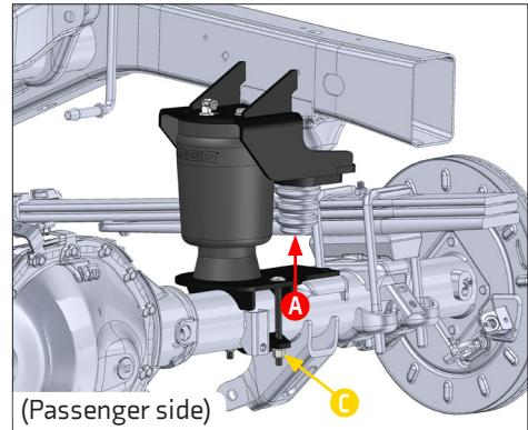
**C** Ensure the lower bracket hasn't shifted and torque the 3/8" hardware to **20 FT.LB.**
