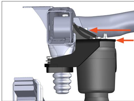
Push the upper bracket against the frame and snug the two 3/8" bolts.
