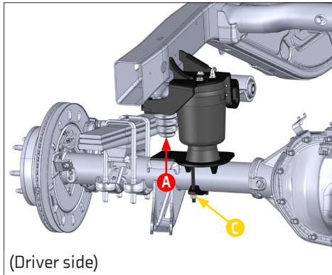
**A** Torque Upper bracket first. Torque the M10 socket head cap screw to **37 FT.LB.** using a 5/16" allen socket.
