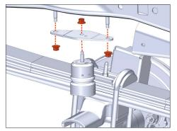
Unbolt factory bumpstop using a 15MM socket.
