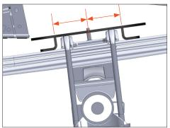
Make sure that the lower bracket is centered Repeat for passenger side. over the U-bolt saddle.
