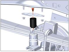
Reinstall factory bumpstop with provided Repeat for passenger side. alumimum spacer and M10 bolt.
