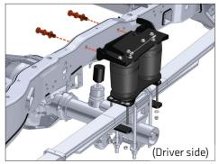
Use the supplied **3.5"** long Grade 8 5/8" bolts, with split washers and flat washers, to attach the upper air spring bracket to the outside of the frame, through the factory sleeved holes. Snug hardware.
