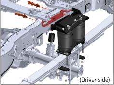
Use the supplied 4" long Grade 8 5/8" bolts, Repeat for passenger side. with split washers and flat washers, to attach the upper air spring bracket to the outside of the hitch, through the factory hitch mounting holes. Snug hardware.
