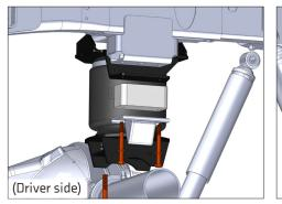
Attach the upper bracket, bump stop spacer, and factory bump stop to the bump stop perch with the supplied M10 bolts and washers as shown.
