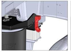
Install the E-brake relocation bracket on the driver side upper bracket using the supplied 1/4" hardware.
