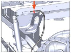
Detach the differential breather line from its anchor point on the frame shown. (On the driver middle of the driver side lower bracket. side of the axle)
