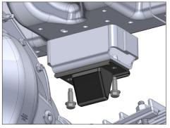
Un-bolt bump stops from both sides of the truck using a 16mm socket.
