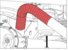
Ensure you have overlap that is about half the thickness of the heat wrap like shown.
