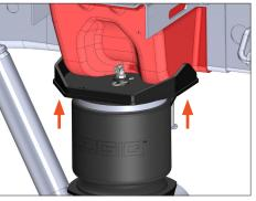
Before snugging the bolts, push the upper bracket up so it is in contact with the crossmember.
