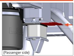
Fill in the gap between the upper bracket and the bump stop perch with as many of the provided shims as necessary.
